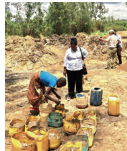
Tanzania has over 6,000 artisanal producers, who make salt by boiling. Water is filtered through a series of pots filled with salt-bearing soil. The resulting brine is concentrated and evaporated to get salt. Significant amounts of this salt reach the market uniodized.
